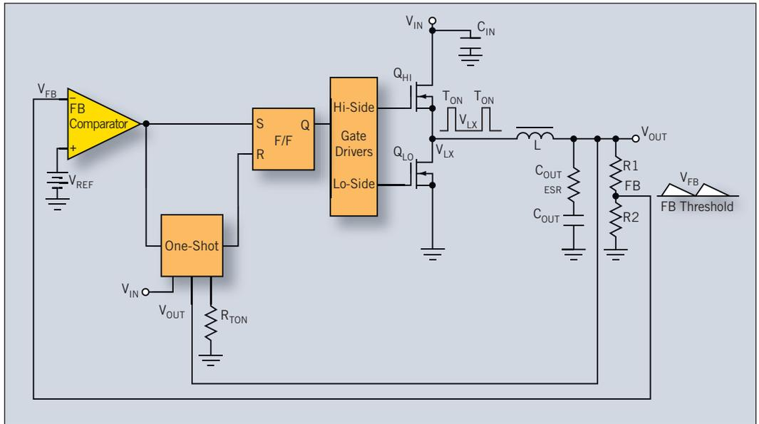
the valley of the output ripple voltage. This ripple voltage is the sum of the two voltages: one produced by the ESR of the output capacitor, and the other due to capacitive charging and discharging of the output capacitor during the switching cycle. For most applications, the output capacitor dominates total output ripple voltage.
