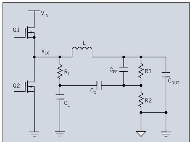
3. Signal injection circuit provides 10 mVp-p at FB.
