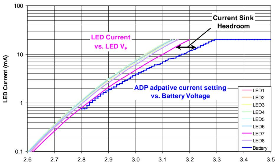
**Figure 2 - ADP Profile as Battery Voltage Decreases (8 LED system)**
