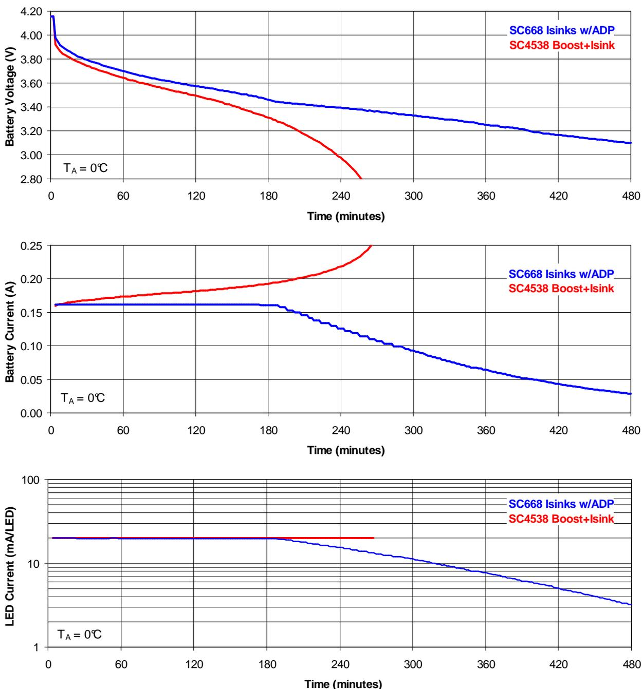
**Figure 9 – Comparison of ADP to Boost Converter LED Driver
