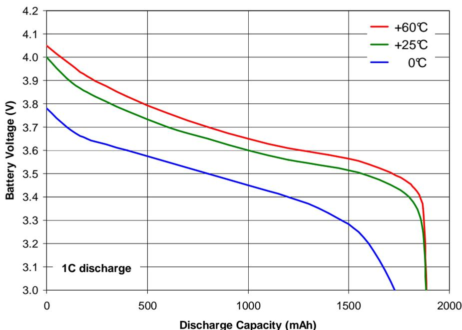
**Figure 6 – Li-ion Battery Discharge Curves vs. Temperature**
