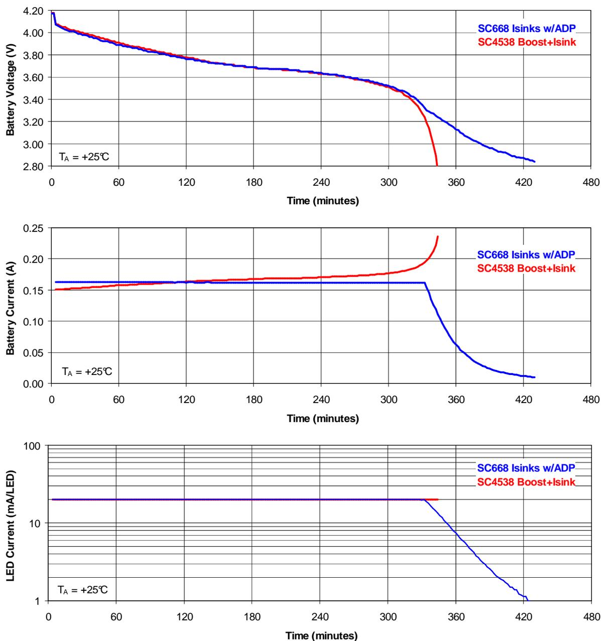
**Figure 8 – Comparison of ADP to Boost Converter LED Driver
