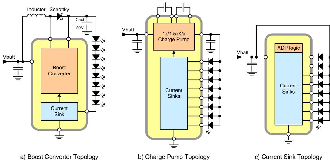
**Figure 1 - White LED Backlight Driver Design Topologies**
