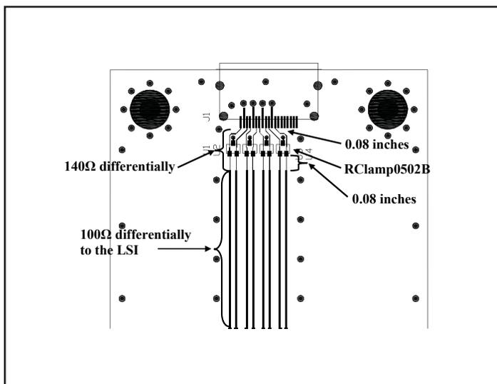
**Figure 3 - HDMI SC-75 Rev D Evaluation Board Design Guideline for RClamp0502B**
