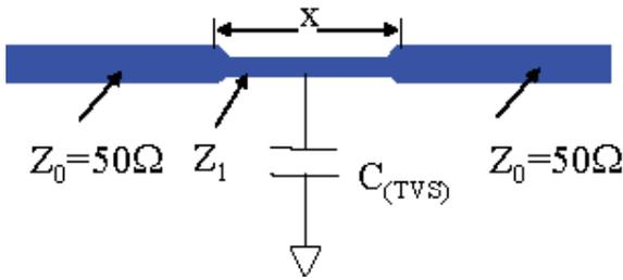
**Figure 1** - Compensation of  $C_{(TVS)}$  with trace length
