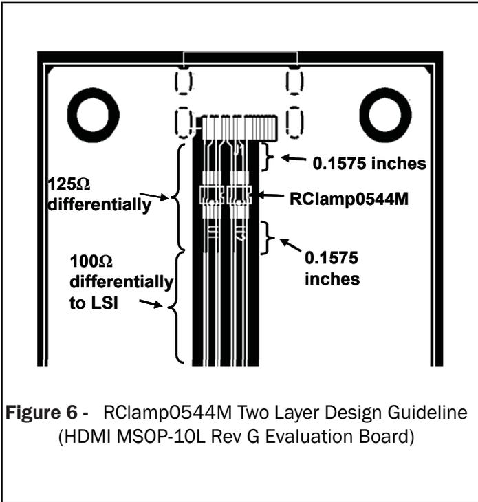
**Figure 6 - RClamp0544M Two Layer Design Guideline (HDMI MSOP-10L Rev G Evaluation Board)**
