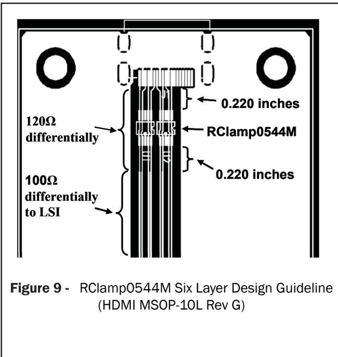
**Figure 9 -** RClamp0544M Six Layer Design Guideline (HDMI MSOP-10L Rev G)
