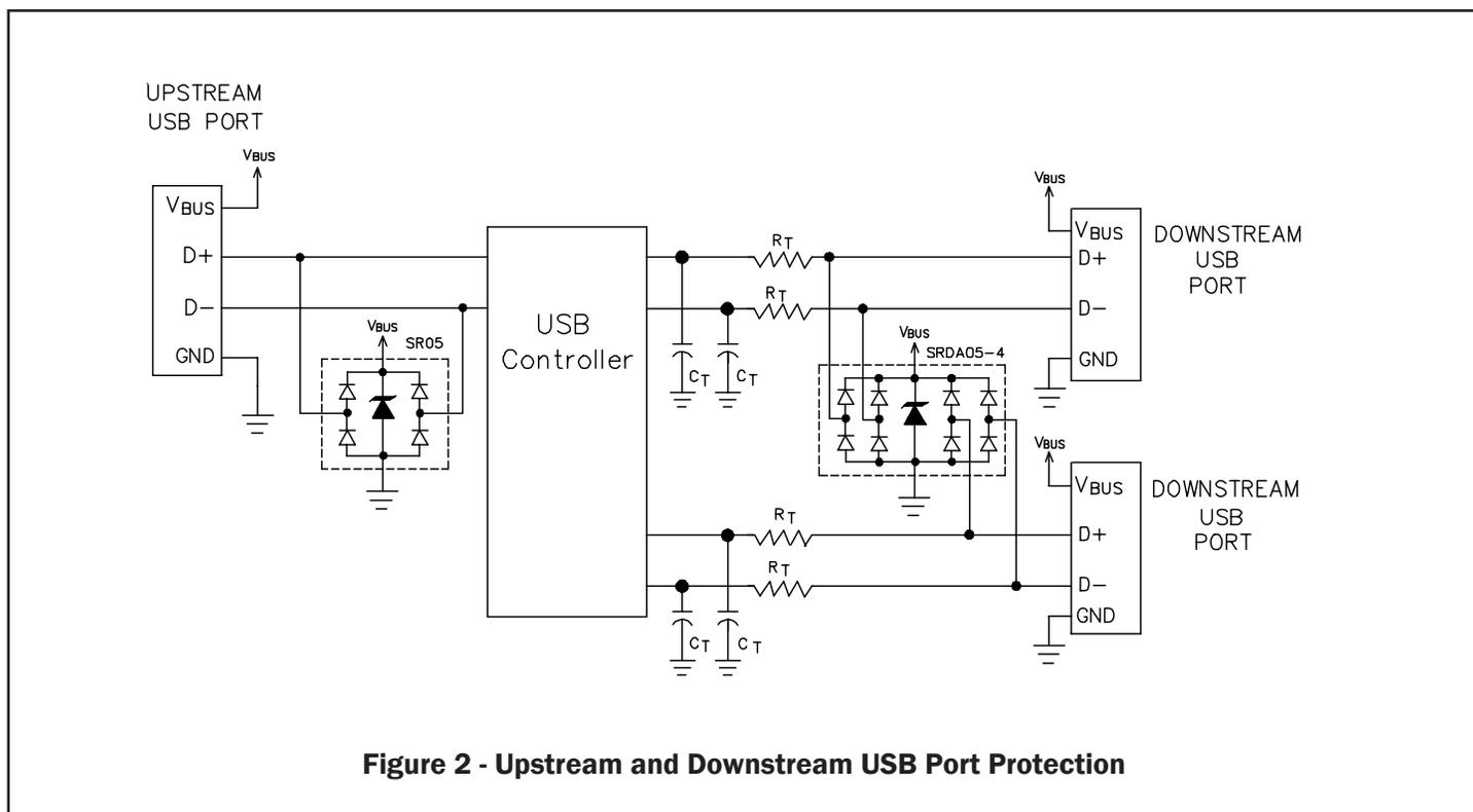
**Figure 2 - Upstream and Downstream USB Port Protection**
