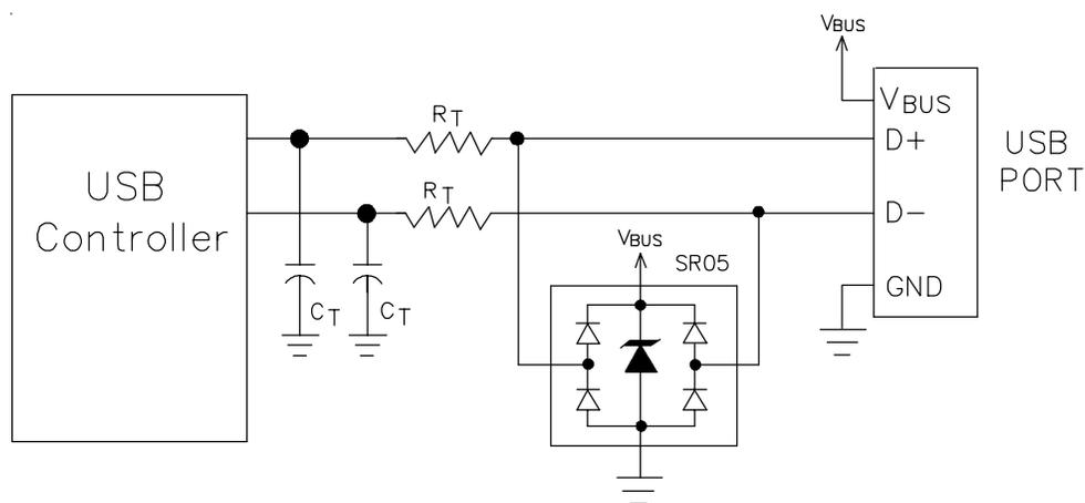
**Figure 1 - Single Port USB Protection**
