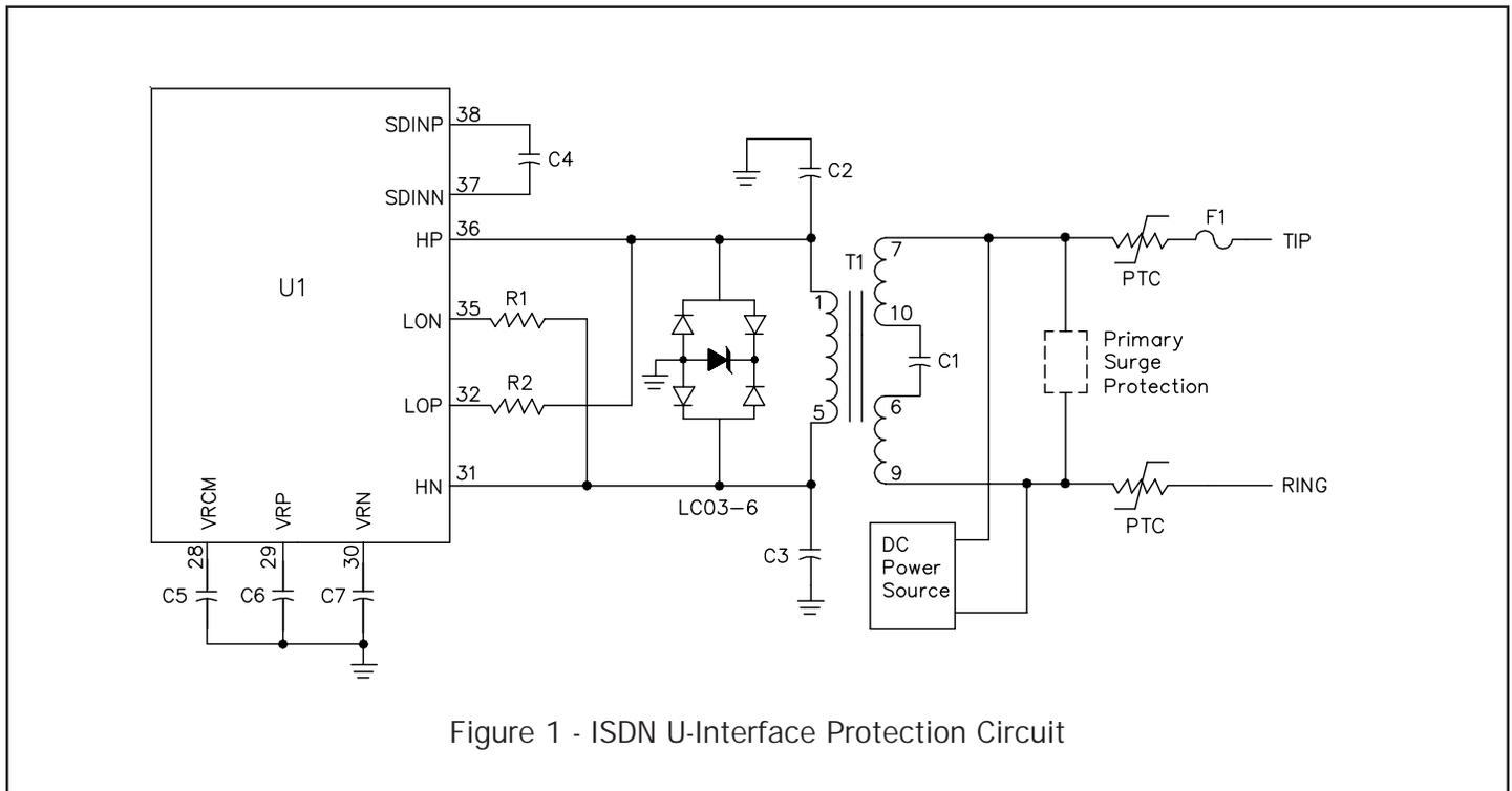
Figure 1 - ISDN U-Interface Protection Circuit
